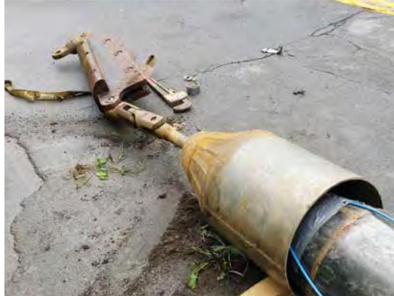
*Cutter Tooling and Expander Head Assembled*
