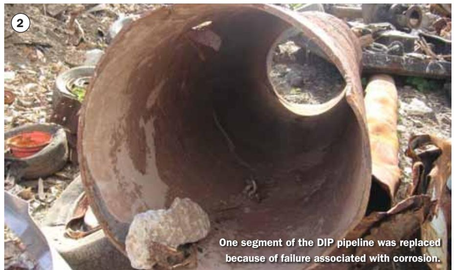
2 One segment of the DIP pipeline was replaced because of failure associated with corrosion.
