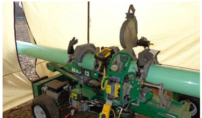
Fusion machine inside cold weather tent
