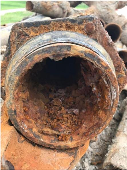
Figure 6: Water main Condition on 6<sup>th</sup> St S.
