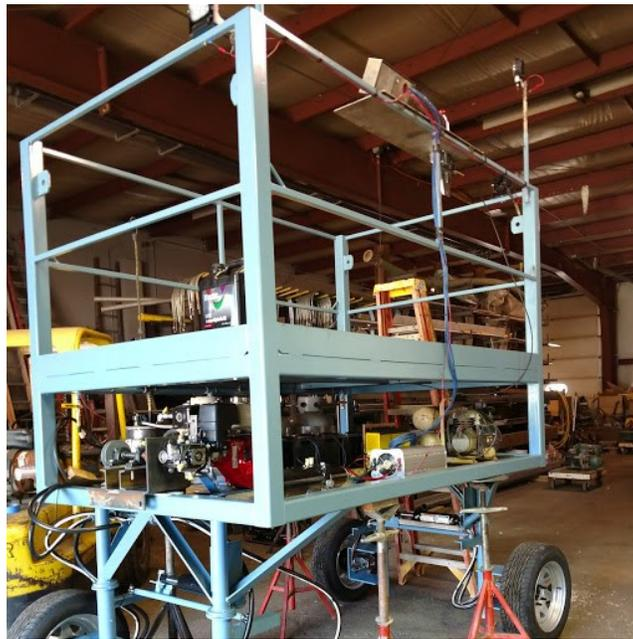
Figure 7. Custom built motorized cart to aid workers in pipe installation inside the 12-foot wide by 14-foot tall trunk sewer.
