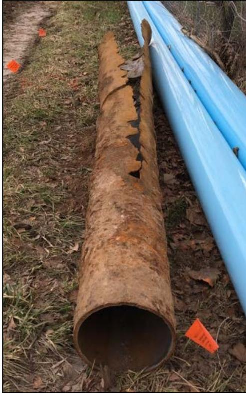
Figure 3. Section of existing ductile iron pipe.
