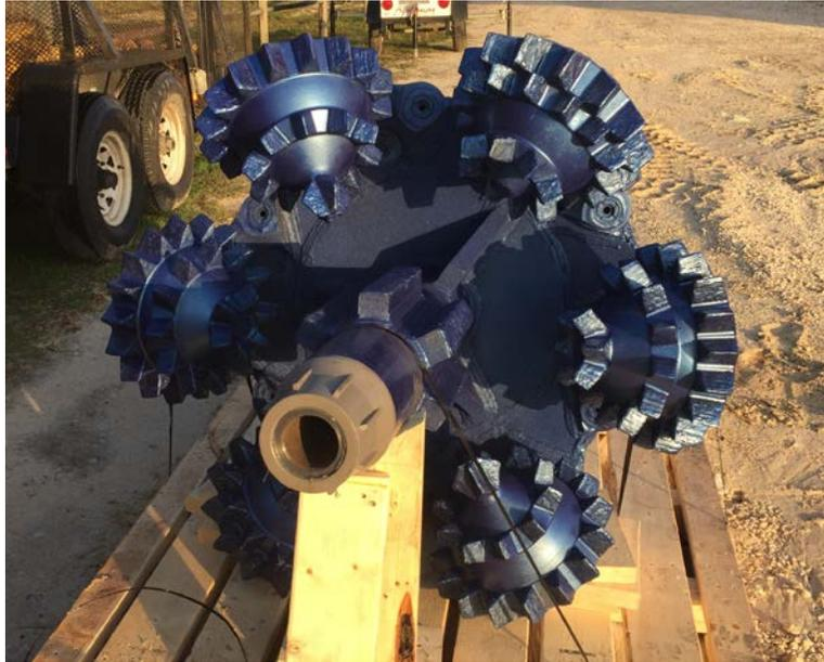
Figure 7. Custom 48-inch tricone drill bit ordered by TB Landmark for the Bay County project.
