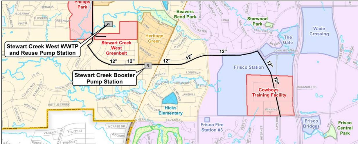
Figure 2. Project vicinity map for reuse pipeline.
