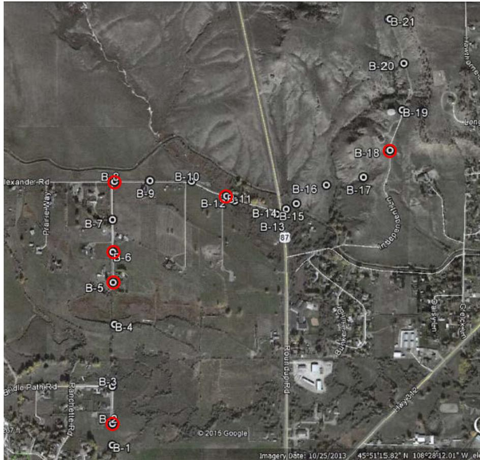
Figure 2. Field exploration map with boring locations along the pipe alignment.
