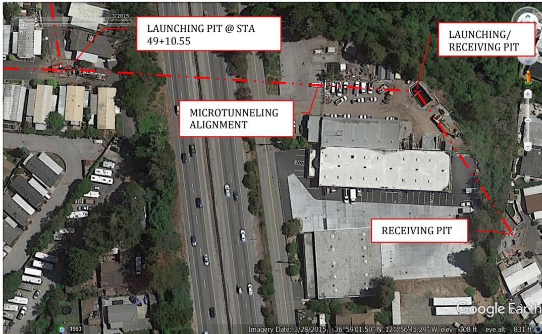
Figure 5. Highway 1 microtunneling crossing
