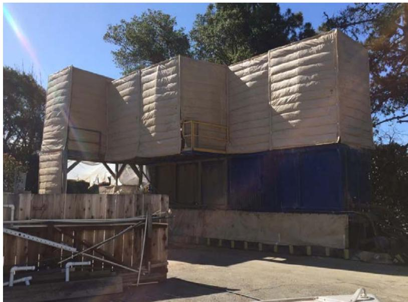
Figure 8. Sound attenuation blanket around microtunneling drilling mud dewatering equipment
