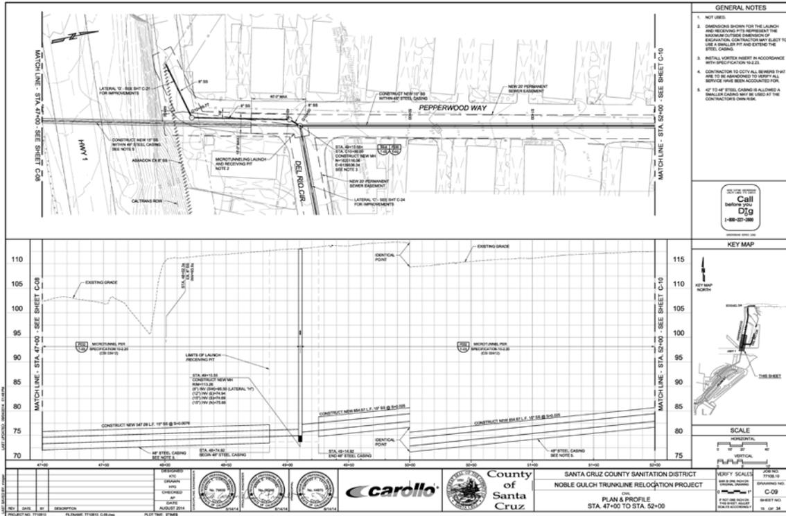
Figure 4. Plan and Profile of one of the deep launching pits
