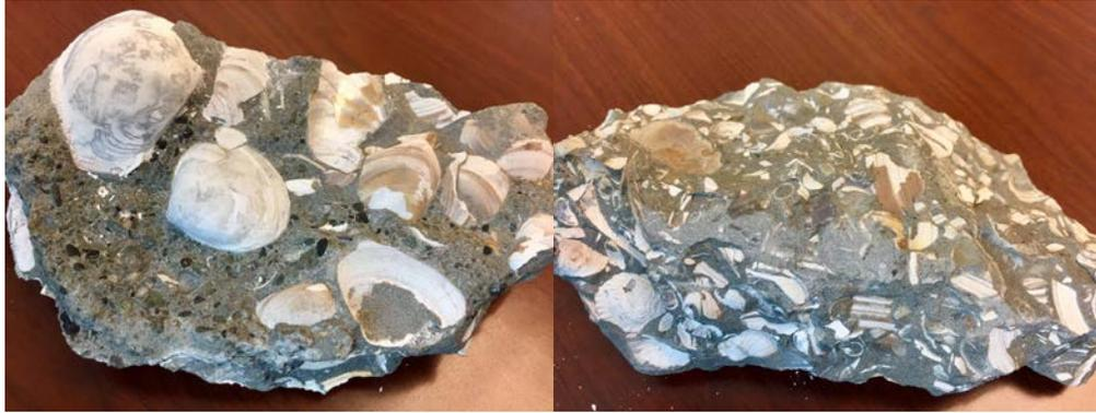
Figure 1: Fossiliferous limestone (nature's concrete) encountered in deep excavations
