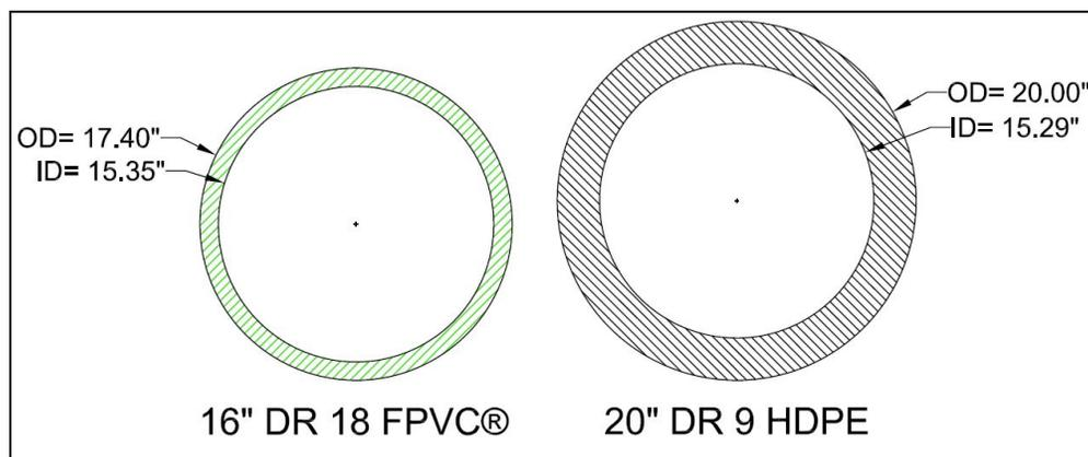
Figure 2. Comparison of 16-inch DR-18 FPVCP and 20-inch DR-9 HDPE IPS cross-sections.
