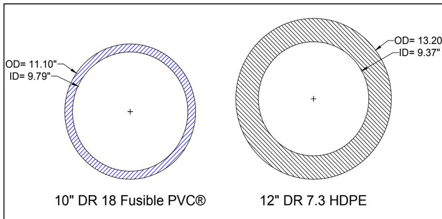
Figure 4. Proposed pipe sizes for Fusible PVC<sup>®</sup> and HDPE
