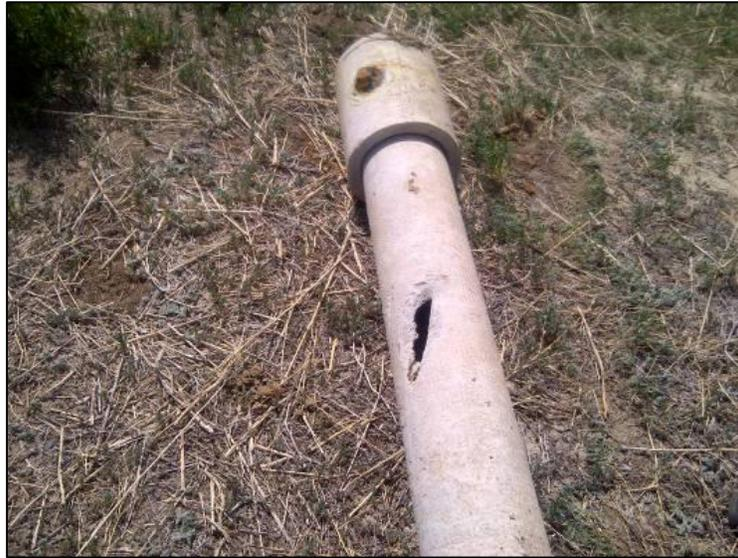
Figure 2. Longitudinal crack along the 6 inch AC pipe.
