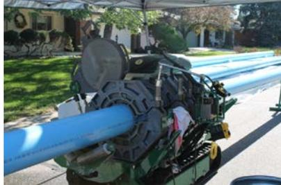
**Figure 10 - Fusible PVC Pipe**
