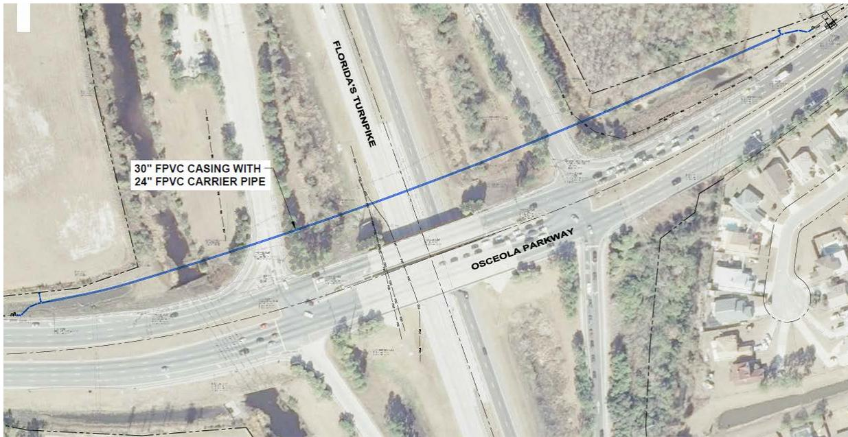
Figure 1. Characterization of the project layout in reference to the Florida Turnpike. The HDD installation took place along the blue alignment shown.
