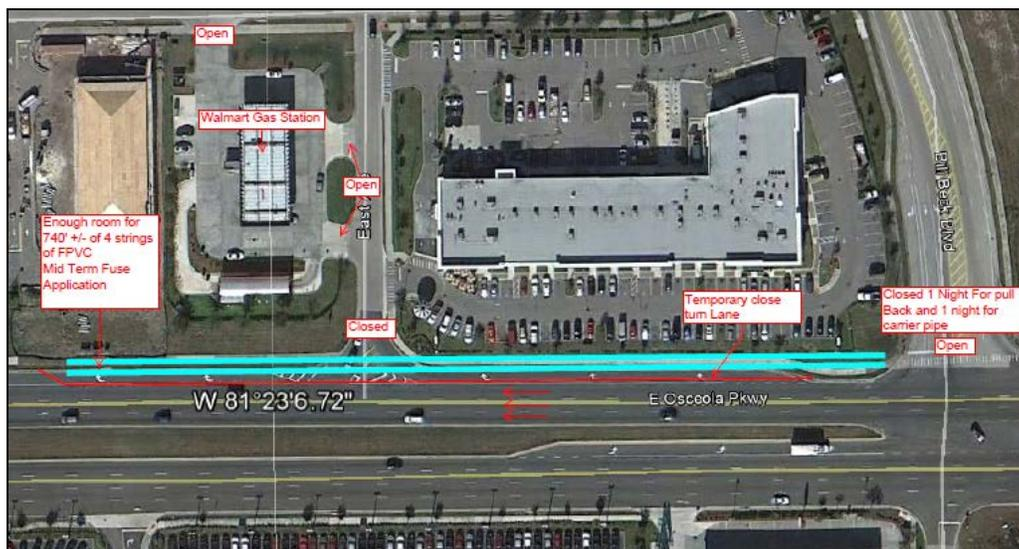
Figure 3. Pipe fusion and laydown area as proposed and then utilized by Andrew Sitework. Two lengths of 30-inch FPVCP and two lengths of 24-inch FPVCP were staged as shown. During the insertion of each pipe, one intermediate fusion joint was performed to create a single length of each pipe. Bill Beck Boulevard, shown on the right side of the picture was closed temporarily during the insertion and intermediate fusion activities.
