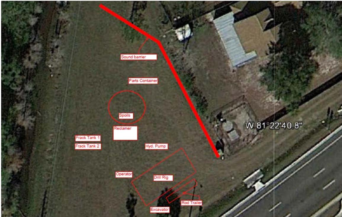
Figure 4. The drill rig operation site is shown in this schematic, based on the revised location proposal and actual location used by Andrew Sitework and the driller, ADS. This is located on the east side of the crossing. Note the location of the sound barrier used to mitigate potential noise issues at the revised drilling location.
