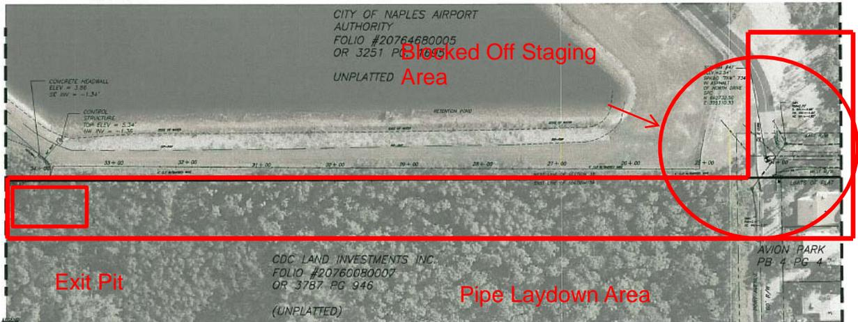
Figure 2. HDD Exit Pit and Staging Area Provided to Contractor for Long Bore
