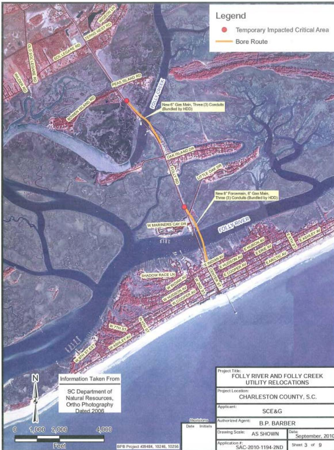
Figure 1. General location and scope of project is shown, including two separate bore locations spanning Folly Creek and Folly River.
