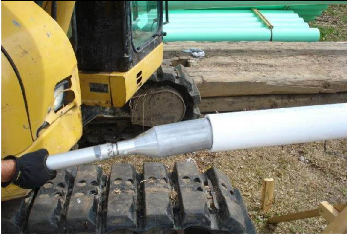
Figure 6. Pipe mandrel used to confirm the internal diameter of the pipe after debanding.
