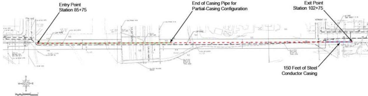
Figure 5. Highway 163 Crossing HDD Bore Plan View
