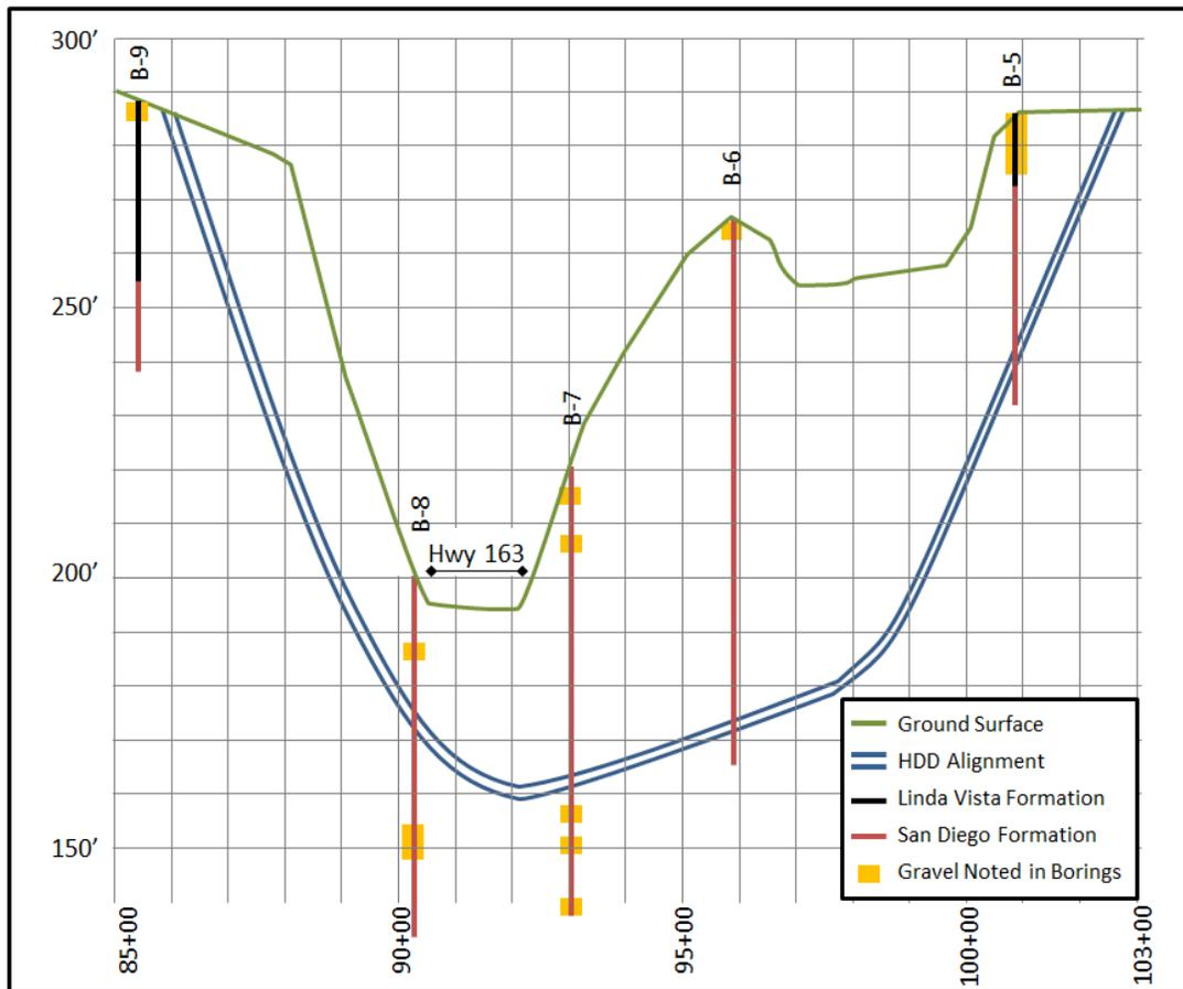
Figure 3. Geotechnical Conditions
