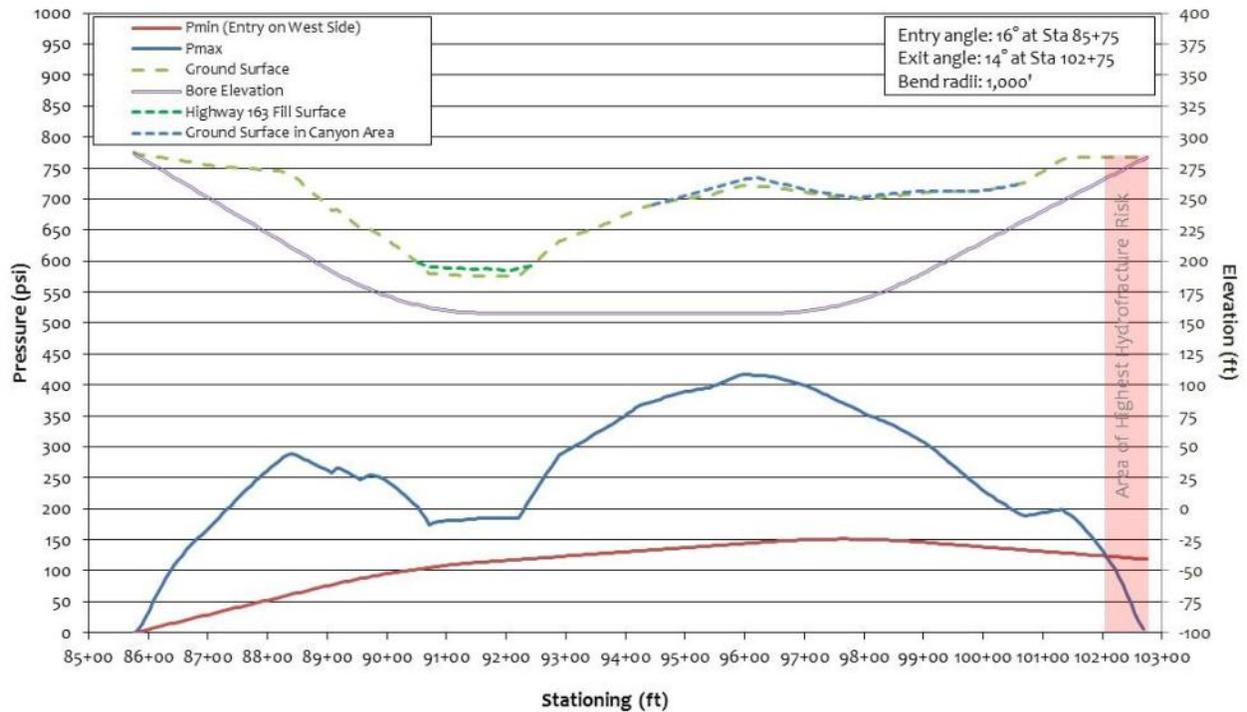
Figure 9. Evaluation of Hydrofracture Risks - Comparison of Maximum Allowable and Minimum Required Drilling Fluid Pressures for the Pilot Bore of the CA Highway 163 Crossing
