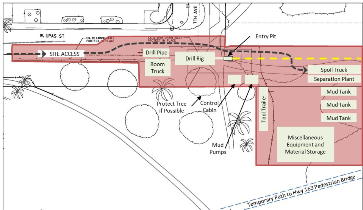
Figure 6. HDD Entry (Rig) Side Work Area and Example Layout (Shaded Area)
