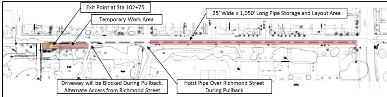
Figure 8. HDD Pipe Layout and Work Area
