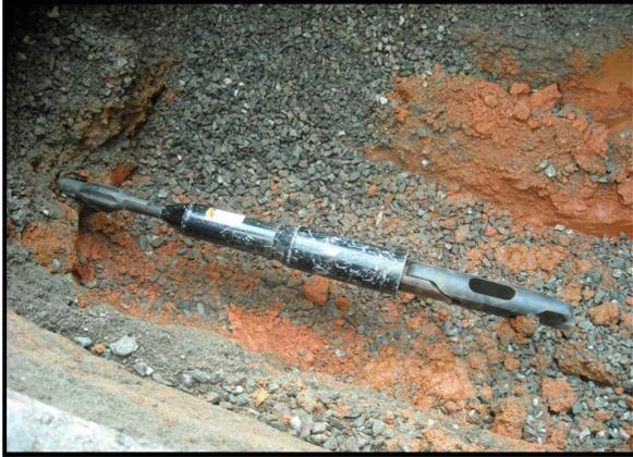
Cutter wheel, 4-inch expander head, and 3-inch rod
