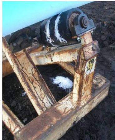
Figure 6. Example of pipe rollers used.
