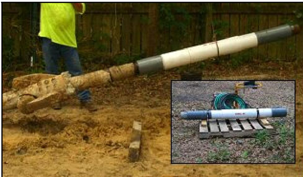
Figure 3. In-line Pull Force Measuring Device
