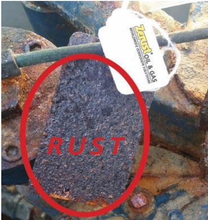
6 week test sump with NO Zerust inhibitor.
