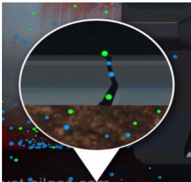
Inhibitors neutralize contaminants on contact and in the vapor space of the annulus. The amount of VCI required depends on the volume of the annulus and any contaminants that may be present.
