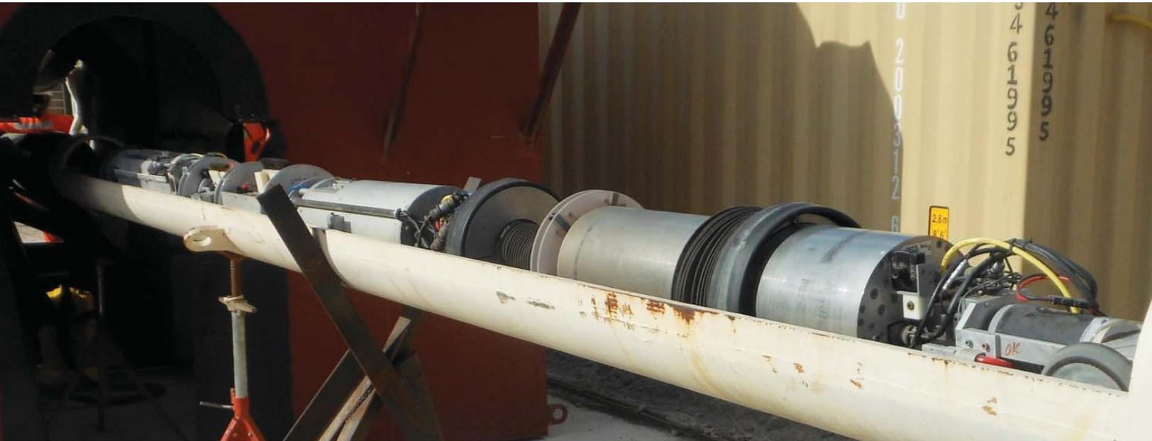
For over 30 years, Aegion Coating Services' robotic technology has strengthened typical corrosion prevention methods by cleaning, coating and inspecting internal field joints in new pipelines. Applying corrosion prevention coatings helps provide end-to-end corrosion protection for all types of pipelines including natural gas, crude oil, potable water and salt water.
