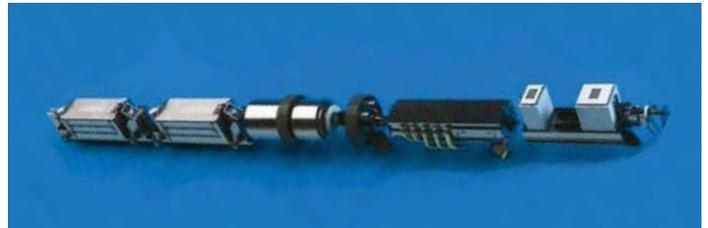
A full train of robotic equipment can apply corrosion prevention coatings to internal field joints.
