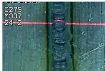
The Inspection Robot features a laser beam that detects unacceptable weld bead contours.
